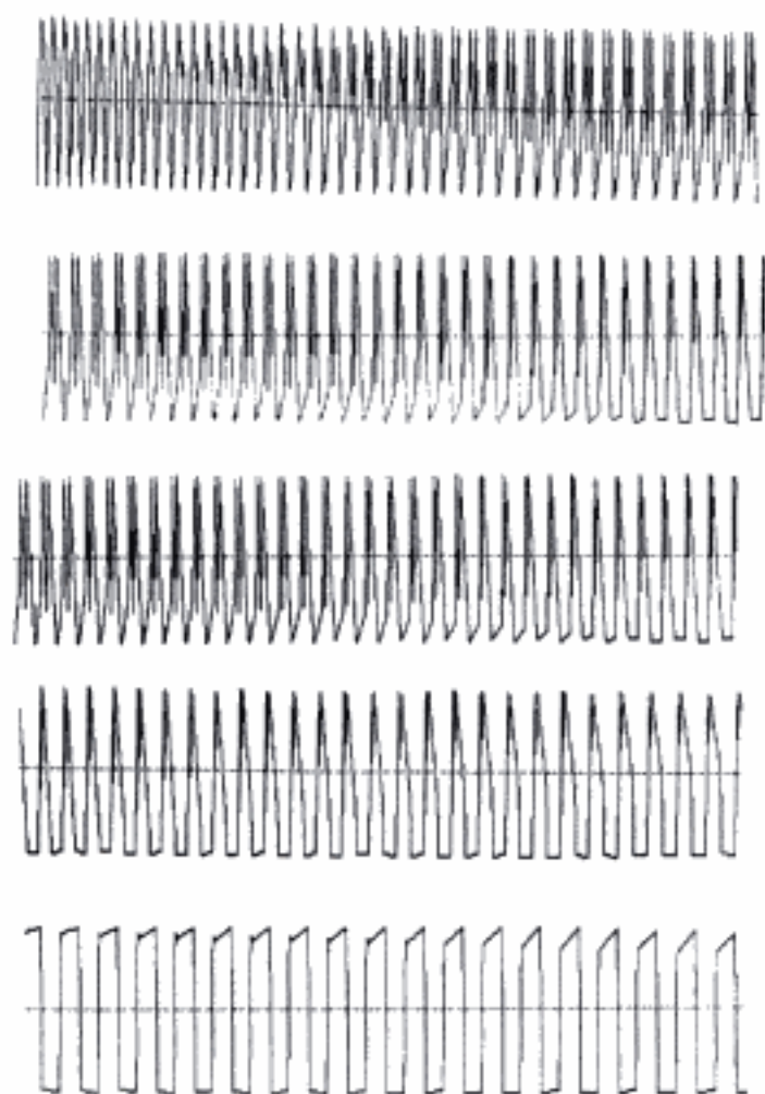
Figure 8.16 Waveform evolution generated by the GENDY program. The progression starts at the top and proceeds to the bottom, plotting time to the right on each line.
